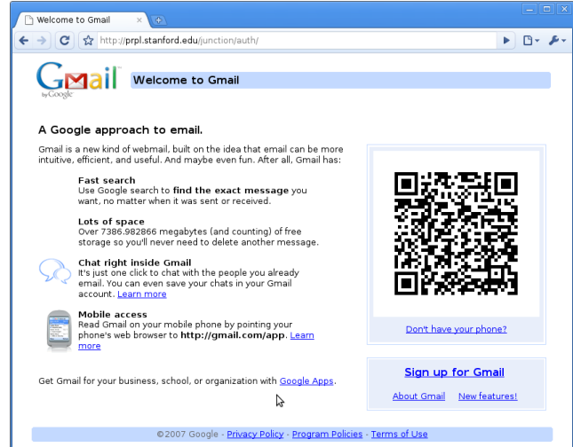
Figure 3. A mock up of a Gmail log-in site using a QR code.
